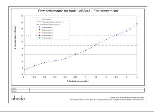
• Min / Max water pressure: 0.75 / 5 bar • Part G mixed flow rate at 3 bar (I/m): 13.36
