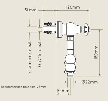
ENSURE CORRECT PRESSURE BEFORE FITTING: Minimum operating pressure 1.0 Bar Recommended operating pressure 2.0 Bar Maximum operating pressure 3.0 Bar
