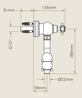
ENSURE CORRECT PRESSURE BEFORE FITTING: Minimum operating pressure 1.0 Bar Recommended operating pressure 2.0 Bar Maximum operating pressure 3.0 Bar
