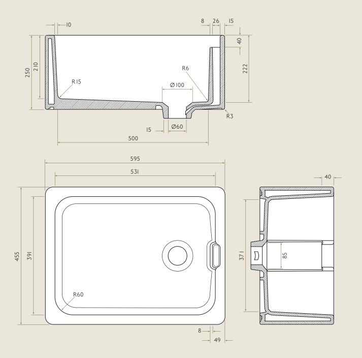
Please note: Sink dimensions are subject to + or - 2% tolerance. All measurements in mm
